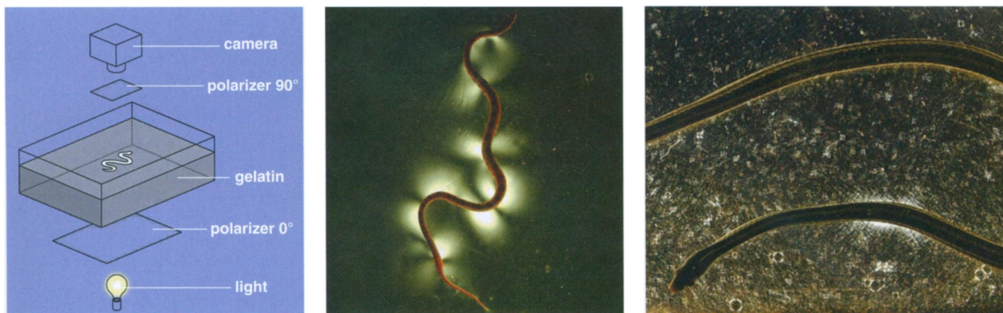
Figure 7. It is difficult to see the pattern of a snake adjusting its weight as it slithers, because the snake's body is often in contact with the ground. One way to visualize regions of higher applied force is to film a snake slithering on gelatin, illuminated from below, between cross-polarizing filters ( left ). The orientation of the filters initially blocks the polarized light from reaching the imager, but when the snake pushes on the gelatin, the light is rotated and can be detected by the camera, as shown by the luminous regions ( middle and right ). Although the adhesiveness of the gelatin can interfere with the snake's natural locomotion, this technique suggests that less of the snake may be in contact with the ground than was previously believed.
