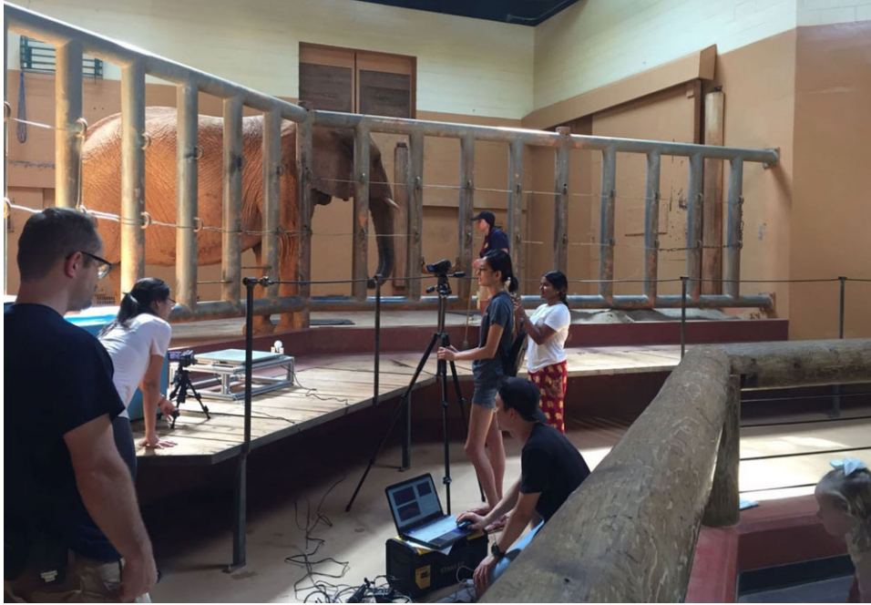
Figure 1. The indoor enclosure where experiments are conducted. During experiments, the elephant turns to face the force plate and video cameras and protrudes its trunk through the enclosure. (Online version in colour.)
