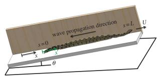
**Figure 2.** Schematic of the apparatus used to study rectilinear locomotion. Here,  $\theta$  is the inclination angle with respect to the horizontal. The front wall (not shown) is composed of Plexiglas. The ground coordinate frame (*x*) and moving coordinate frame (*x'*) are indicated by the arrows. The direction of wave propagation in rectilinear locomotion is opposite to the direction of motion. (Online version in colour.)
